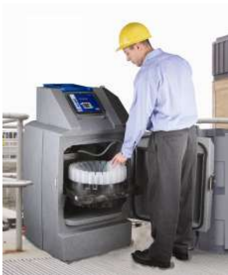
A slide-out bottle rack and swing-away distributor arm allow obstacle-free access to your samples.
