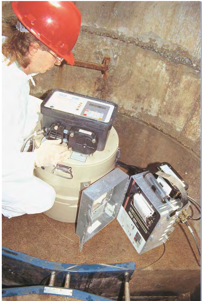
A 4230 Bubbler paces an Isco 3700 Sampler to collect flow proportioned samples.
